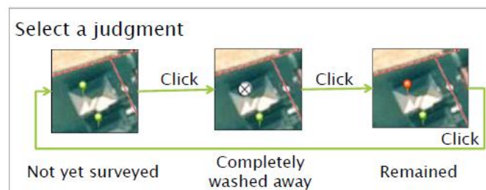
Figure 5. Judgment selection for building damage only by clicking
