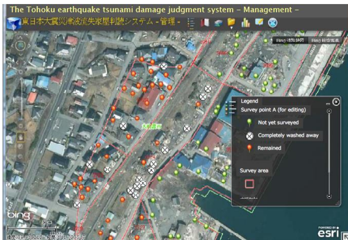
Figure 4. Screen design concept for the washed-away building judgment system using a Web-GIS
